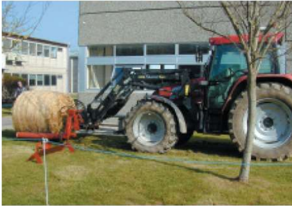
Á Side View of the Modified Bale Handler Attachment with Bale Rotating Feature.
