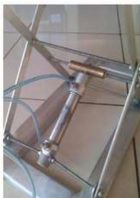
Pneumatic cylinder used with Air Lift and driven by hand
