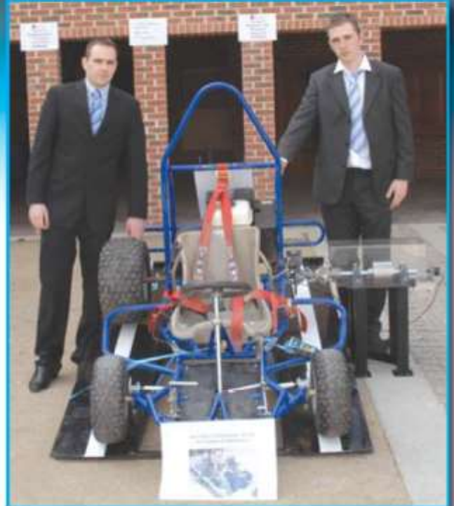
The Kart Chassis Dynamometer design, development and manufacture was carried out in conjunction with the CIT Engine Test Cell Centre.
