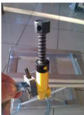
Pneumatic cylinder used with Air Lift and driven by hand
